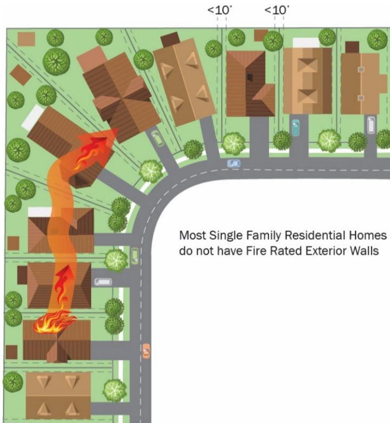
Figure 2. Typical residential building separations (10–20 feet) are vulnerable to structure-to-structure fire spread under extreme wildfire conditions, as most single-family residences have non-fire rated exterior walls.
