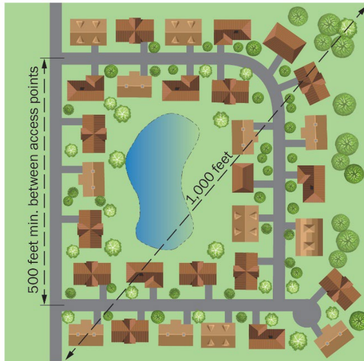
Figure 15. Access roads should have sufficient separation.
