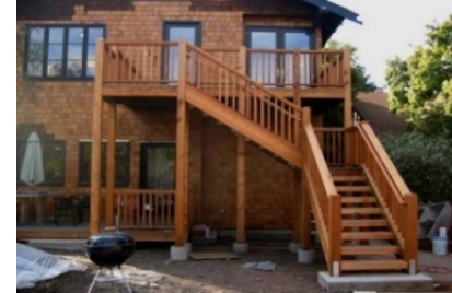
Figure 38: Deck with Single Set of Stairs
