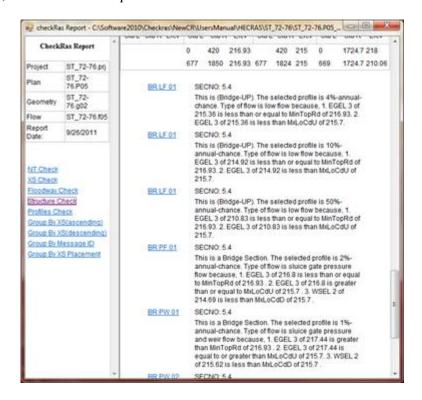
The cHECk-RAS **Report** window will be displayed. Select one of the reports from the left side of the window. The above figure shows the Structure Check Report. The first few messages listed in the report are flow type messages for all the profiles in the flow file, except for the floodway. Using the flagging function in the **Report Editor** window, the user can suppress informational messages such as these.
