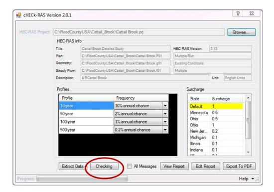
Note that the checking process may take several minutes depending on the size and complexity of the file. Progress can be seen in the Progress bar at the bottom lefthand side of the interface window. Upon completion, a pop-up message will appear indicating that the checking routine has been completed.
