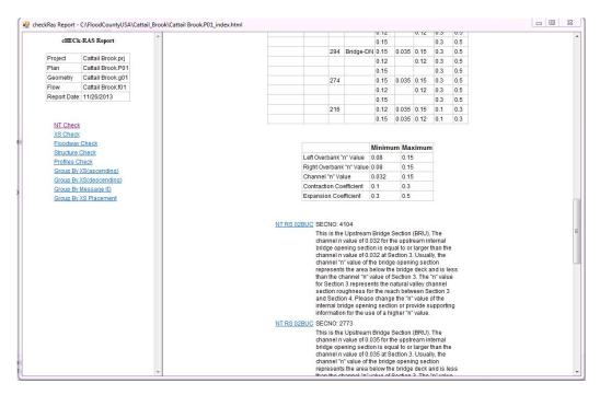
At the top of each report is a summary table of the data extracted from the HEC-RAS project (.prj) file and used by cHECk-RAS in its checking routines. Each message generated by cHECk-RAS that flags a potential issue is listed following the table(s) generated for each type of check. By clicking the hyperlinked **Message ID** to the left of each message, additional Help information for that particular message will display in a separate pop-up window.
