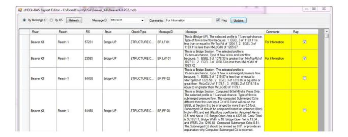
The report can be ordered either by Message ID or by cross section number by using the radio buttons at the top lefthand side of the window and then clicking the Refresh button. By default, the report will be ordered by Message ID.
